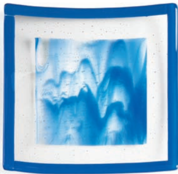
Figure 7 This plate was formed with two separate firings. The first was a full fuse and the second was a slump firing.
