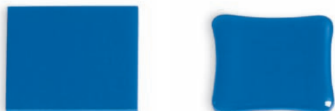
Figure 3: One, 1/8" (3mm) layer fired to 1500°F (816°C). Notice how the edges pull in.
