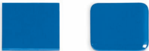
Figure 1: Two, 1/8" (3mm) layers fired to 1500°F (816°C). Notice that the area covered stays the same and the edges are straight.
