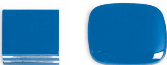
Figure 2: Five, 1/8" (3mm) layers fired to 1500°F (816°C). Notice substantial spread in area.
