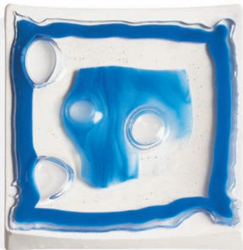
Figure 8 This plate was formed with a single firing for both fusing and slumping. This shortcut caused edge distortion and bubbles.
