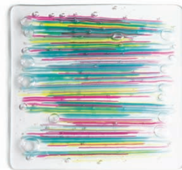
Figure 6 In firing, the edges of this tile sealed, preventing the escape of air bubbles trapped between stringers.
