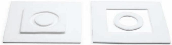
Figure 3a: Positive and negative ceramic fiber paper designs.
