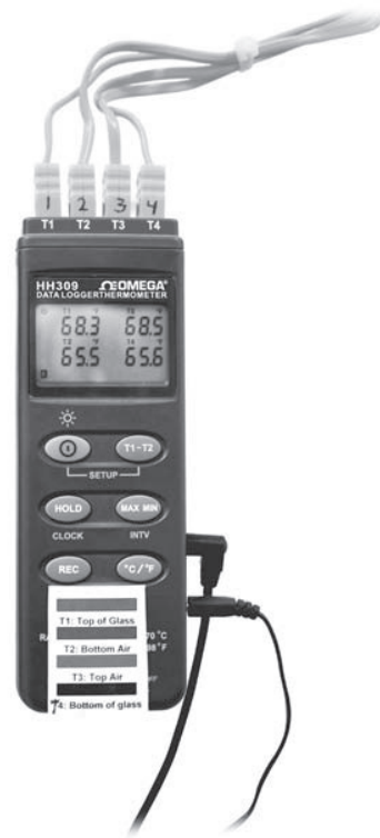
FIGURE 2: SOME PYROMETERS CAN RECORD DATA.
