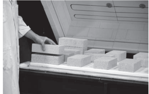
FIGURE 11: WEIGHTING THE FIBERBOARD SHELF WITH BRICKS.
