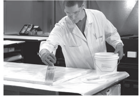
FIGURE 8: BRUSHING QF-180 ONTO THE FIBEROARD SHELF.
