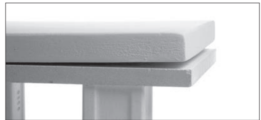
FIGURE 12: EXAMPLE OF A BOWED FIBERBOARD SHELF CORNER.
