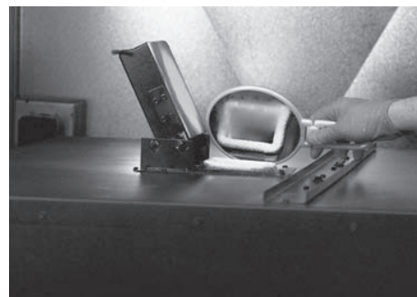
FIGURE 7: USING A MIRROR TO CHECK FOR CONDENSATION.
