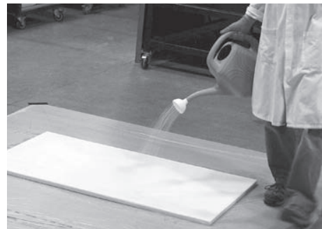
FIGURE 6: A WATERING CAN WITH A SHOWERHEAD SPOUT WILL CONTROL THE FLOW OF COLLOIDAL SILICA.
